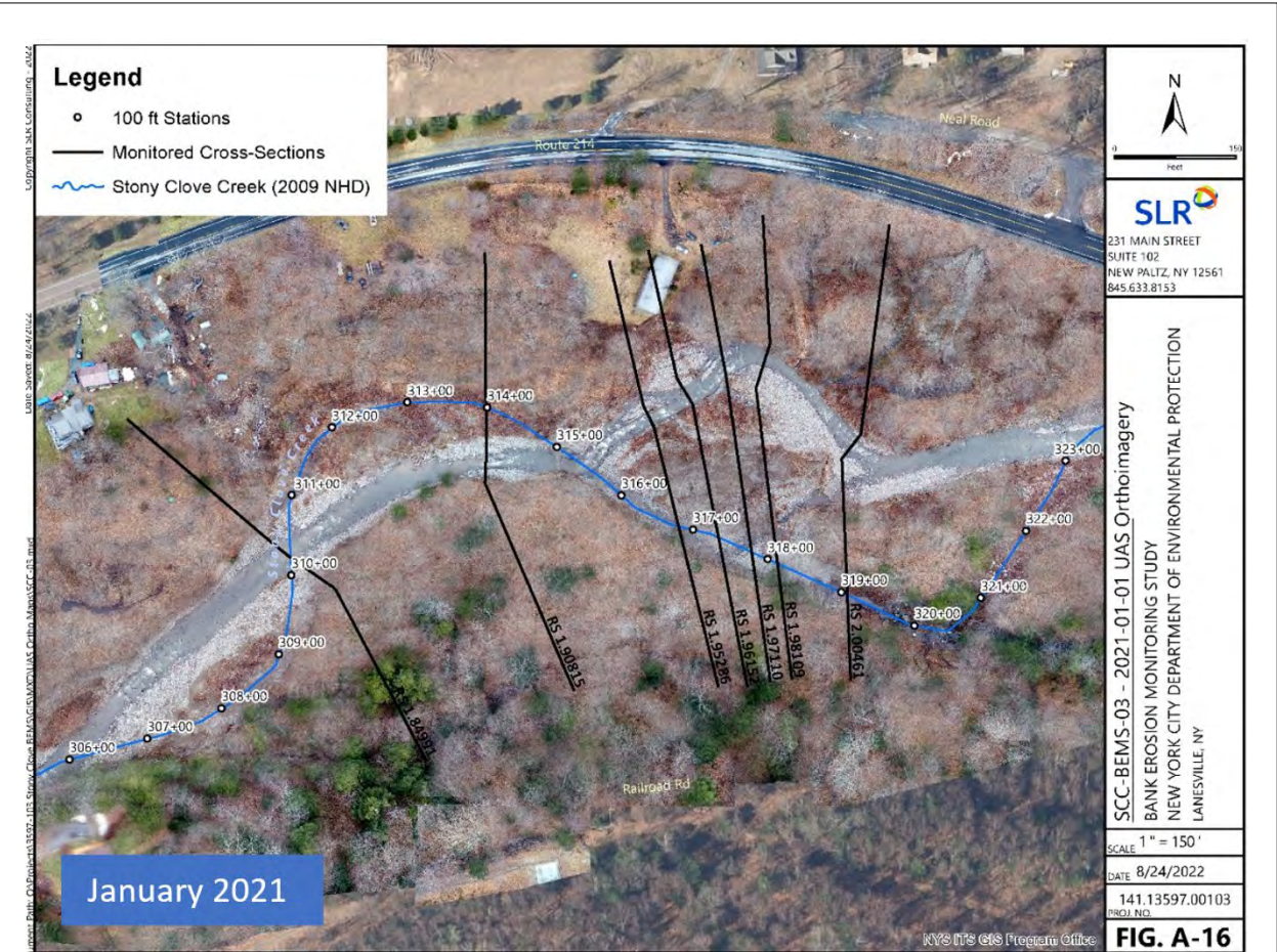
Figure 4.27 SCC-03 January 1, 2021 orthophoto used for SfM derivation of a digital topographic surface for morphologic monitoring and geomorphic change detection following the December 25, 2020 flood. Source: SLR Consulting, 2023.
